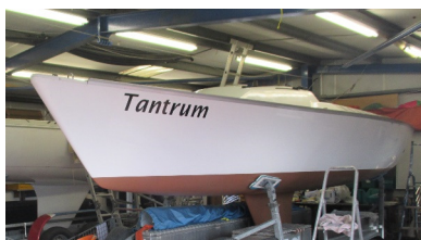
Tantrum with Coppercoat completed
